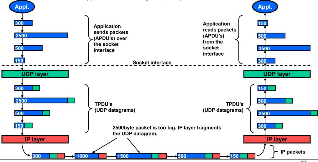
UDP is best suited for applications with short command-response type "transactions" that do not justify the establishment / release prior to the data exchange.
