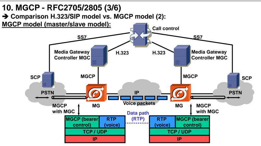
→ The MGCP model is asymmetric: A master (MGC) controls a slave (Media Gateway MG). The MGs do not know the state of a call. They just open voice channels (PSTN side) and RTP streams (IP side) and pass voice between IP and PSTN.
