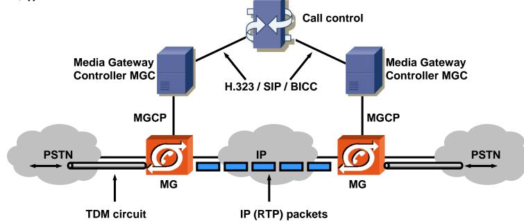
MG: Media Gateway (converts from voice in TDM circuit to RTP (IP) packets). MGC: Media Gateway Controller (controls MG via MGCP protocol). Call control: Central control of call. Call control box controls MGC boxes via H.323 or SIP.
