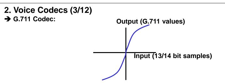
The G.711 Codec performs compansion (COMPression and ExpANSION) for reducing the data rate and amplify weak signals in order to increase S/N ratio:
