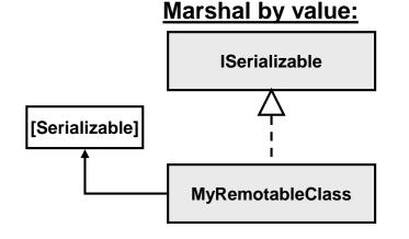
The attribute Serializable is attached to MyRemoteClass marking it serializable (all members of the class need to be serializable as well). Optionally MyRemotableClass may implement the ISerializable interface allowing custom serialization.
