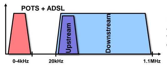
Upstream and downstream use overlapping frequency bands, but the signals are separated with an echo canceller.
