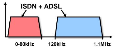
ISDN's and ADSL's frequencies are overlapping, thus ADSL and ISDN frequency bands need to be separated (ADSL with out-of-band ISDN does not use frequencies in ISDN band).
